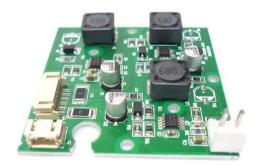
Pcb (LED-driver) PML-80 (SL-COB80-3CC)
