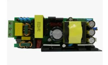
Pcb (Power supply) V1: 36V/3A V2: 12V/1A LED PFE-60 WW Profile Spot (LPD-120-36/12)
